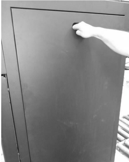
Figure 14 – Removal of side covers
